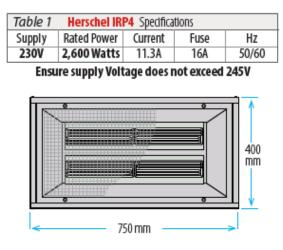
Wiring to this unit must be connected in accordance with the relevant national electrical safety standards and must be earthed. The electrical supply to the unit should be provided by connecting to a circuit protected by a fuse or miniature circuit breaker suitable for the electrical rating of the unit and in accordance with Table 1.
