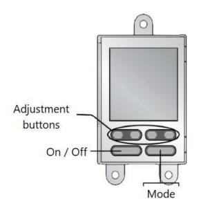
The TDI Thermostat is used to control the Ecostrad Ecowarm.
